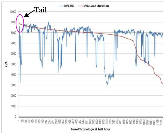
Fig. 3 kVA data with load duration curve-small tail
