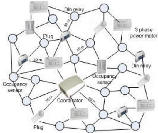
Fig. 5 ZigBee mesh network with ZigBee devices
