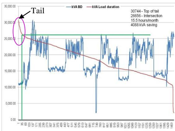
Fig. 4 kVA data with load duration curve-large tail
